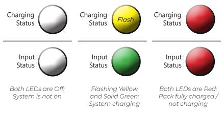
If both lights are red, it indicates the system is not charging. This can be caused by the following:
